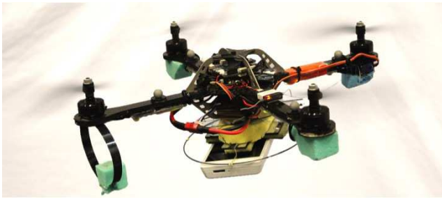
Fig. 16. The downwards-facing gripper can also be used to carry payloads such as this cell phone.
