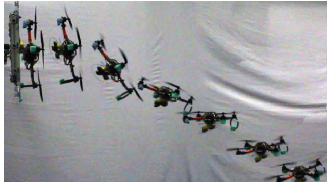
Fig. 14. A strobe of images from a perch sequence. The robot starts on the right hand side outside of the field of view, accelerates towards the target, and rotates in time to achieve a successful perch within the landing envelope of the gripper.
