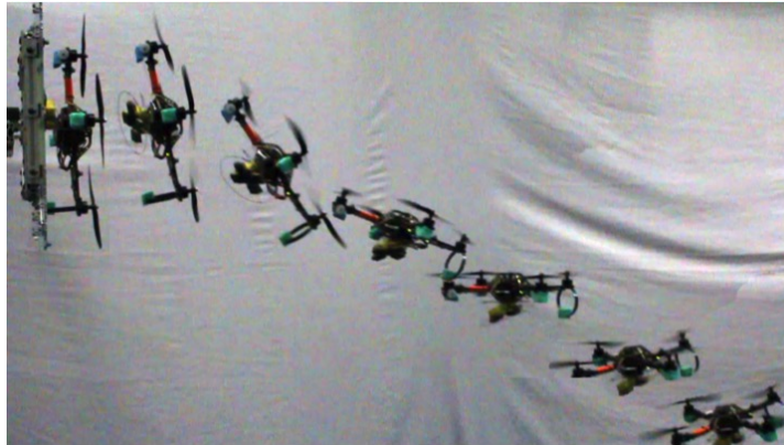
Figure 4.14: A strobe image sequence of a perching robot. The robot starts on the right hand side outside of the field of view, accelerates towards the target, and rotates in time to achieve a successful perch within the landing envelope of the gripper.
