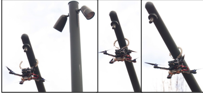
Figure 5.1: A sample outdoor perch location for a quadrotor on a cantilevered cylindrical light post. Note that the axis of the cylinder can generally be oriented.
