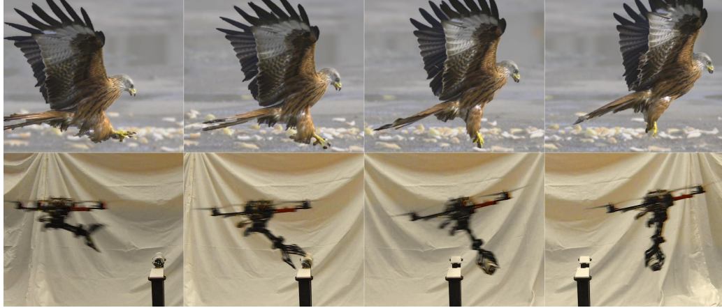
Figure 3.9: A still image comparison between a raptor (red kite, extracted from [124]) and the quadrotor for a trajectory with the quadrotor moving at 3 m/s (9 body lengths / second) at pickup. See [130] for a video of the grasping.
