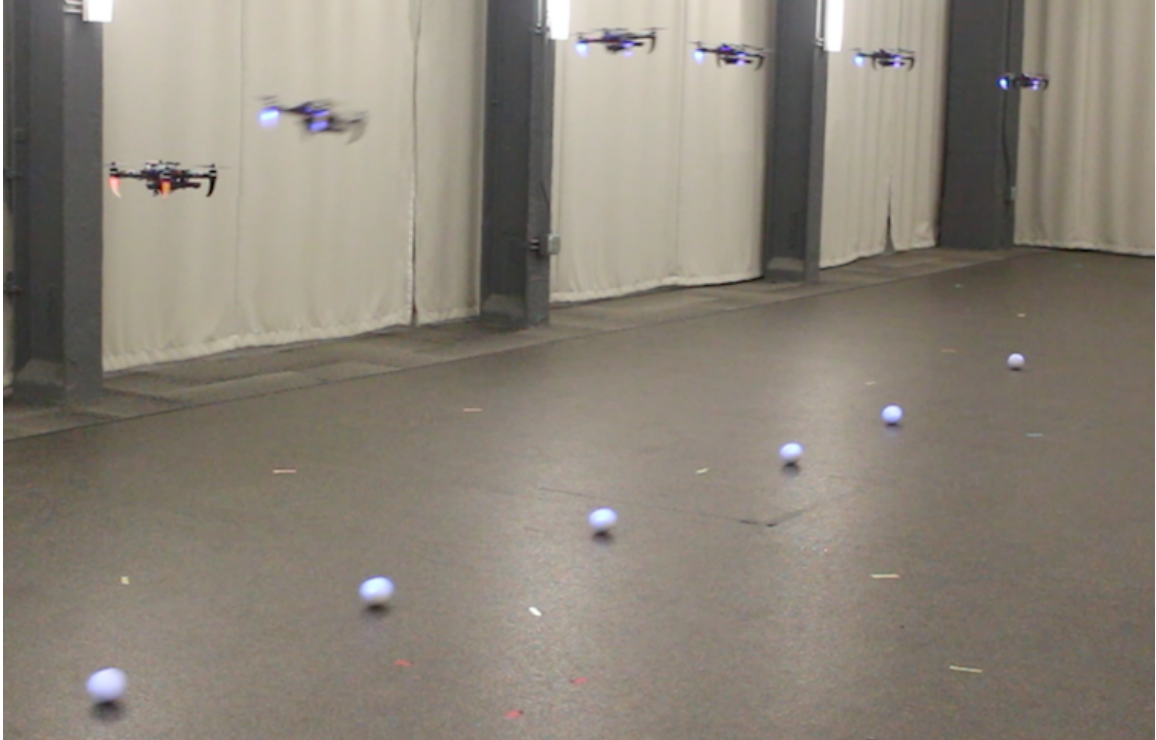
Figure 6.15: A quadrotor accelerates to track a target moving at 1.5 m/s. The motion is planned in real time and considers the estimated trajectory of the target, the dynamics of the robot, the actuator limitations, and the camera's field of view. All sensing and computation occurs onboard the robot and leverages only one downward-facing camera and an onboard inertial measurement unit.
