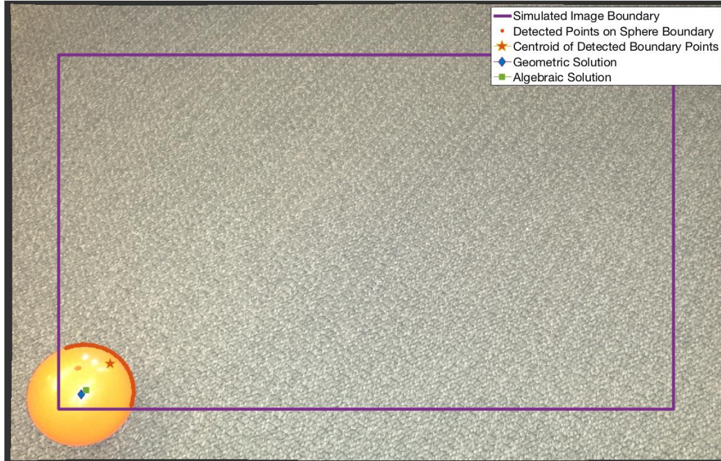
Figure 6.2: A sample comparison between sphere detection approaches. The purple frame indicates a simulated image boundary. Red circles denote detected boundary points of the sphere. In this case, more points were actually detected, but points outside of the simulated image boundary were discarded. The centroid of the remaining points is represented by the red pentagram. The computed bearing to the center of the sphere using the geometric solution is denoted by the blue diamond, and the computed bearing to the center of the sphere using the algebraic solution is denoted by the green square. In this case, the centroid does not accurately represent the bearing to the center of the sphere. The geometric solution is best, but it requires more computation time.
